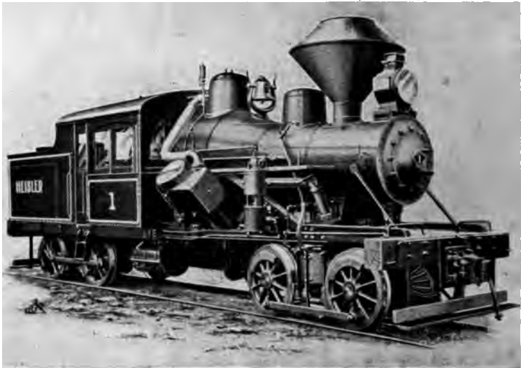
FIG. 87. — A Heisler Geared Locomotive.
